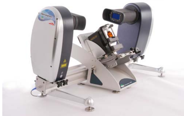
Figure 1: Malvern Spraytec system for the characterization of nasal pump sprays.
