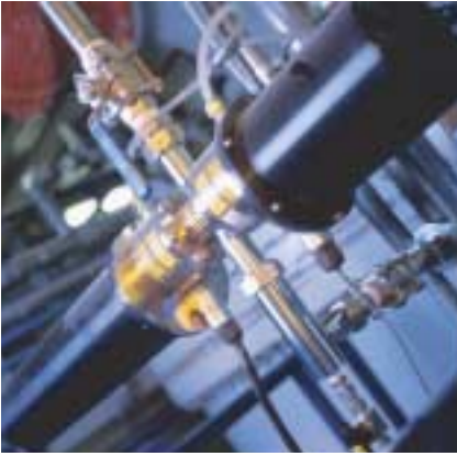
A close-up view of the particle size analyzer. A venturi, right, aspirates each sample before measurement to duplicate the velocity of particles in process flow.
