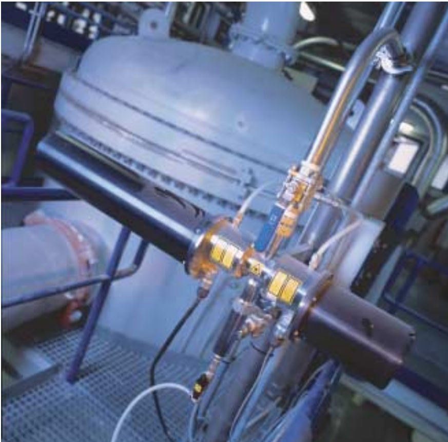
The on-line particle size analyzer, installed between the mill and a blending silo, constantly withdraws samples from the pneumatic conveying line for measurement. It then returns the sample to the flow of product.
